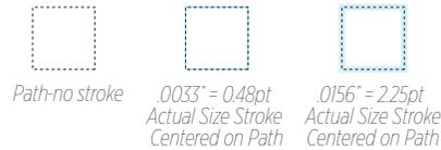
Traps range between .0033" to .0156" depending on the substrate and intended printed content.
